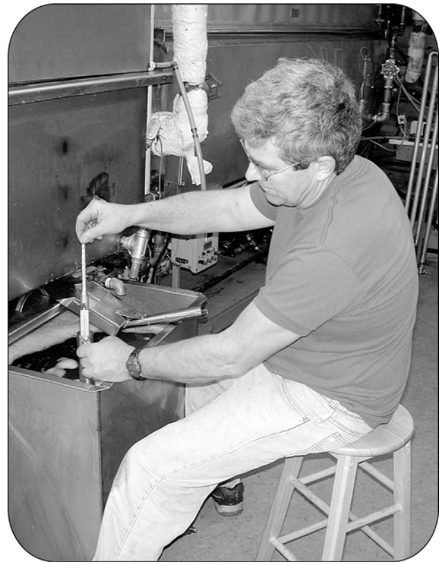
Figure 2. The observed Brix value can be read directly on the Brix scale on the hydrometer stem.
