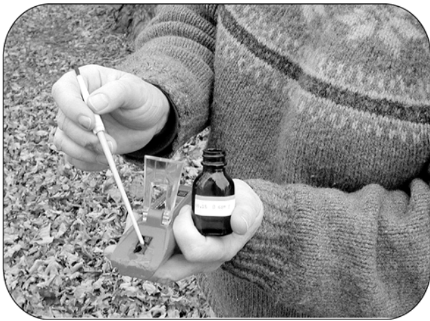
Figure 5. Spread the oil or syrup sample evenly across the glass prism with a plastic rod or stir stick.
