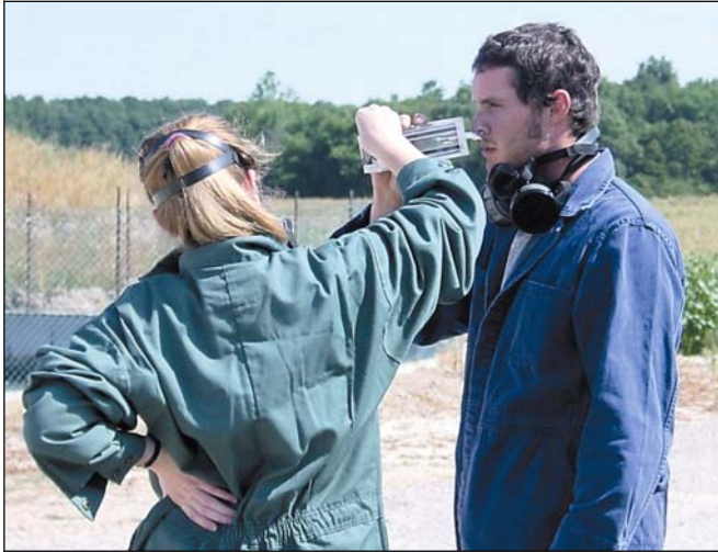
Figure 7. Researchers involved in odour testing with large livestock operations use a scentometer to measure manure odour levels at various distances from a barn.
