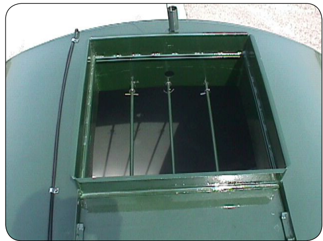
Figure 3. Safety hatch for liquid manure tanker.
