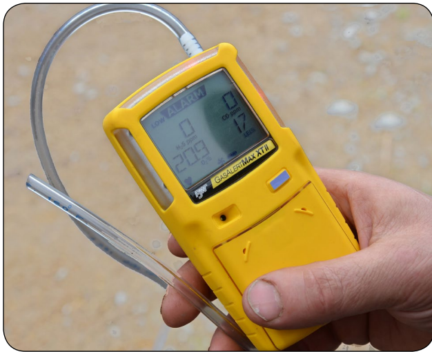
Figure 2. Example of handheld multi-gas detector used to monitor concentration of oxygen, hydrogen sulphide and explosive gas (% LEL — Lower Explosive Limit) available at safety supply stores.
